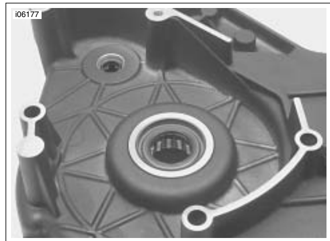
Figure 4. Oil Seal Properly Installed in Inner Primary Housing
